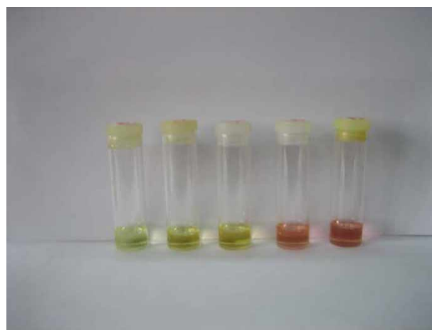
FIGURE 3 The color change of compound 1 ( 1.0 \times 10^{-5} M in DMSO) after addition of different amounts of F^- . From left to right: free, +25.0 equiv, +45.0 equiv, +70.0 equiv, + OH^- .
